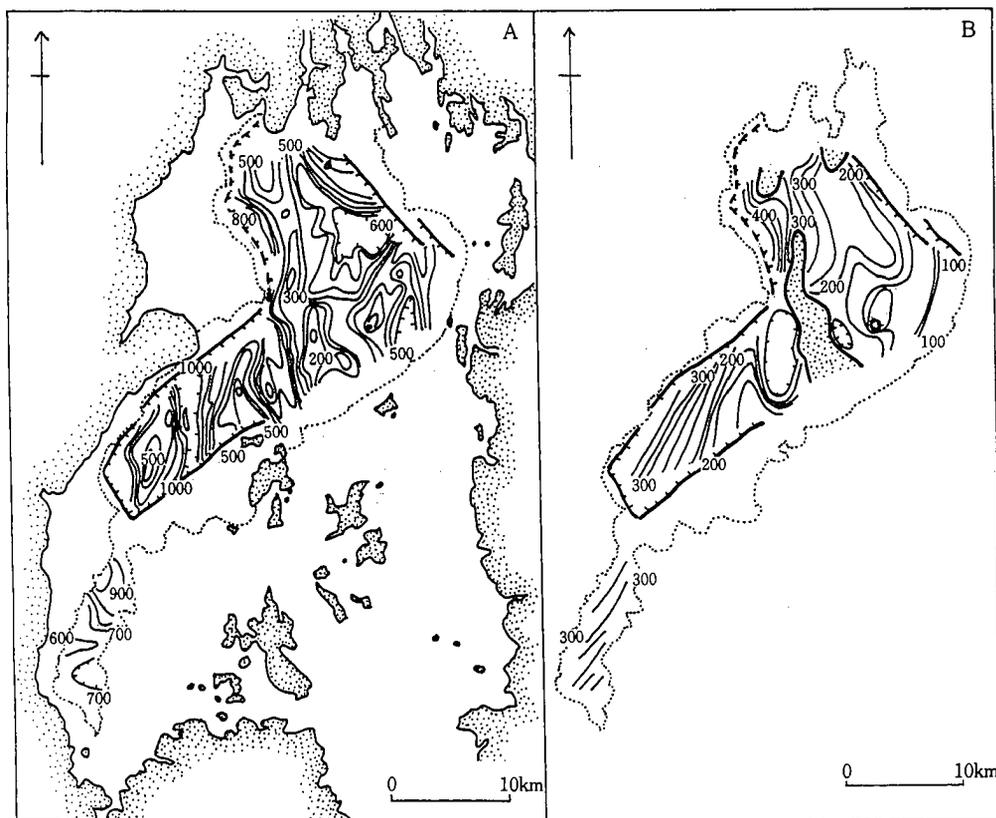
Fig. 6 Isopach contour maps of BB (A) and TS (B) reflection surfaces.
