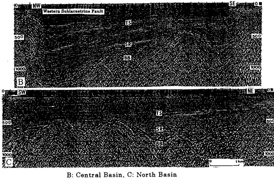
Fig. 5 Seismic profiles of B and C lines by air gun method. B line is crossing the central basin, C line is crossing the north basin. Survey lines are shown in Fig. 3.
