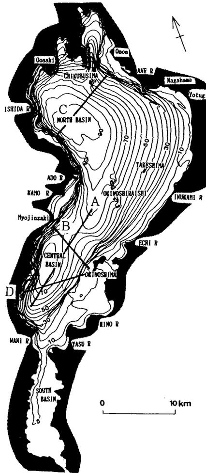
Fig. 3 Bathymetric chart of Lake Biwa, and survey lines of air gun (A, B and C) and uniboom (D) Contour interval: 5 m.
