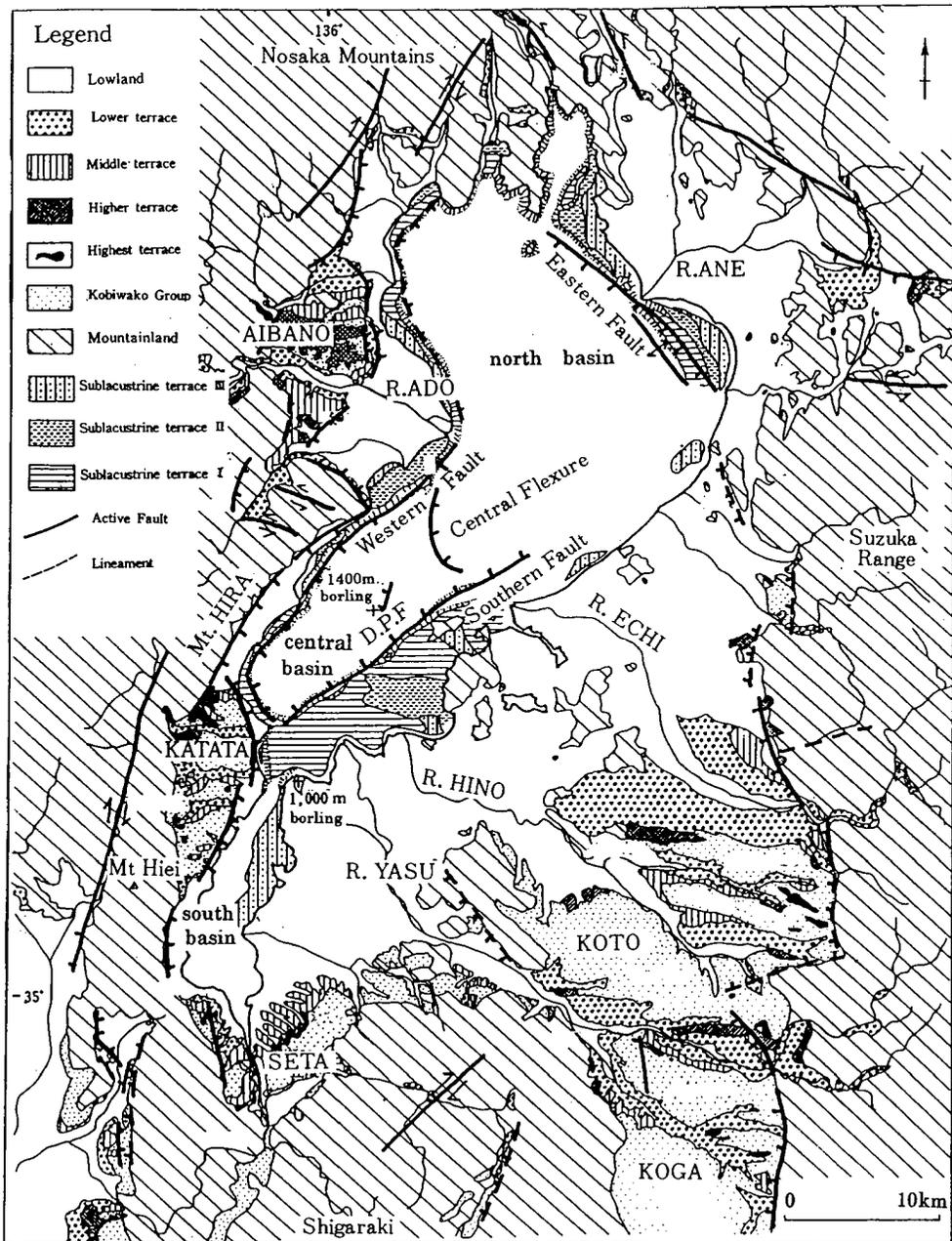
Fig. 2 Distribution of terrace, sublacustrine terrace and active faults of Lake Biwa and its surroundings. DPF : Drilling point fault
