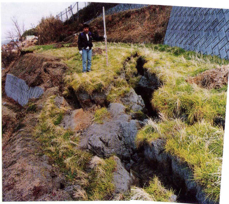
写真6. 地点⑬. 江崎における断層と地表変位の連続 Photo. 6 Trace of surface rupture occurred in paddy field near Loc ⑬, looking the south
