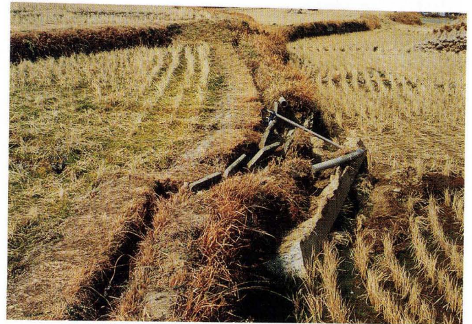
写真46. 地点㉕. 畦の変位状況 Photo. 46 Right lateral offset of footpath at Loc ㉕
